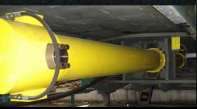
9" main-ram cylinder with up to 286,277 lbs. of platen force delivers up to 40% more force than competitive balers using 9" cylinders.
