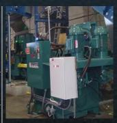
Never get caught empty handed with a blown fuse! Electrical panel employs service friendly molded case and mini circuit breakers for all circuits both main and branch.\*
