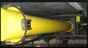
8" main-ram cylinder with 211,000 lbs of platen force delivers up to 40% more force than competitive balers using 8" cylinders.
