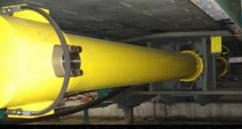
11" main-ram cylinder with 427,649 lbs. of platen force delivers up to 30% more force than competitive balers using 11" cylinders.
