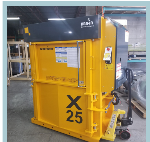
Low overall installed height (<6.5 ft.) due to the internal crossed cylinders.
