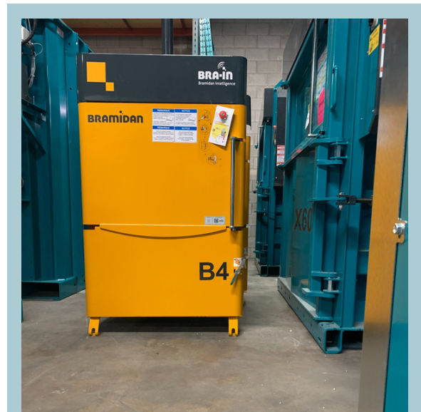
Frontal Tie System allows the baler to be placed up against a wall.
