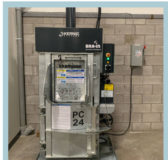
Frontal Tie System allows the baler to be placed up against a wall.
