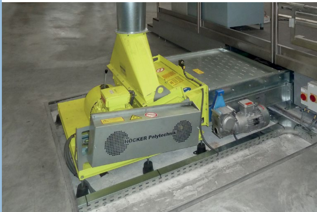
PHSS-K/B shredder Disposes die cutting waste and lateral front waste.
