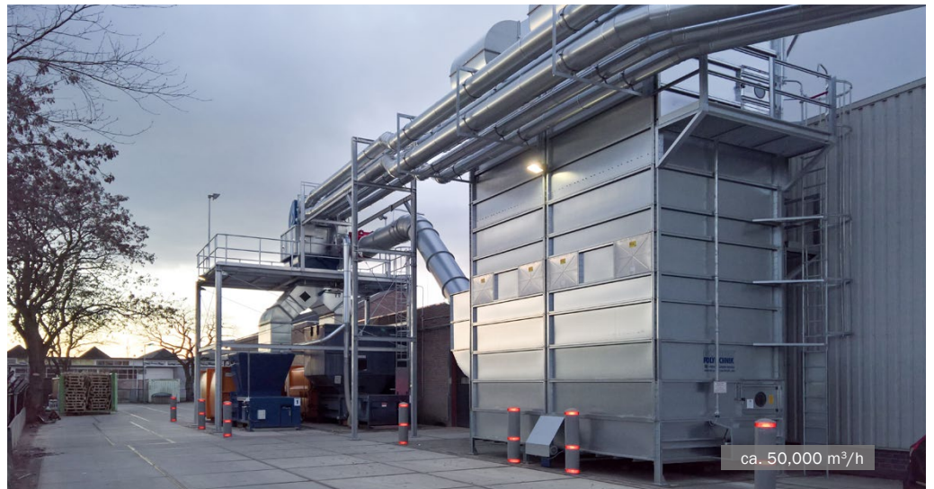
MultiStar sliding bar filter with mit jet cleaning • printing and packaging industry
