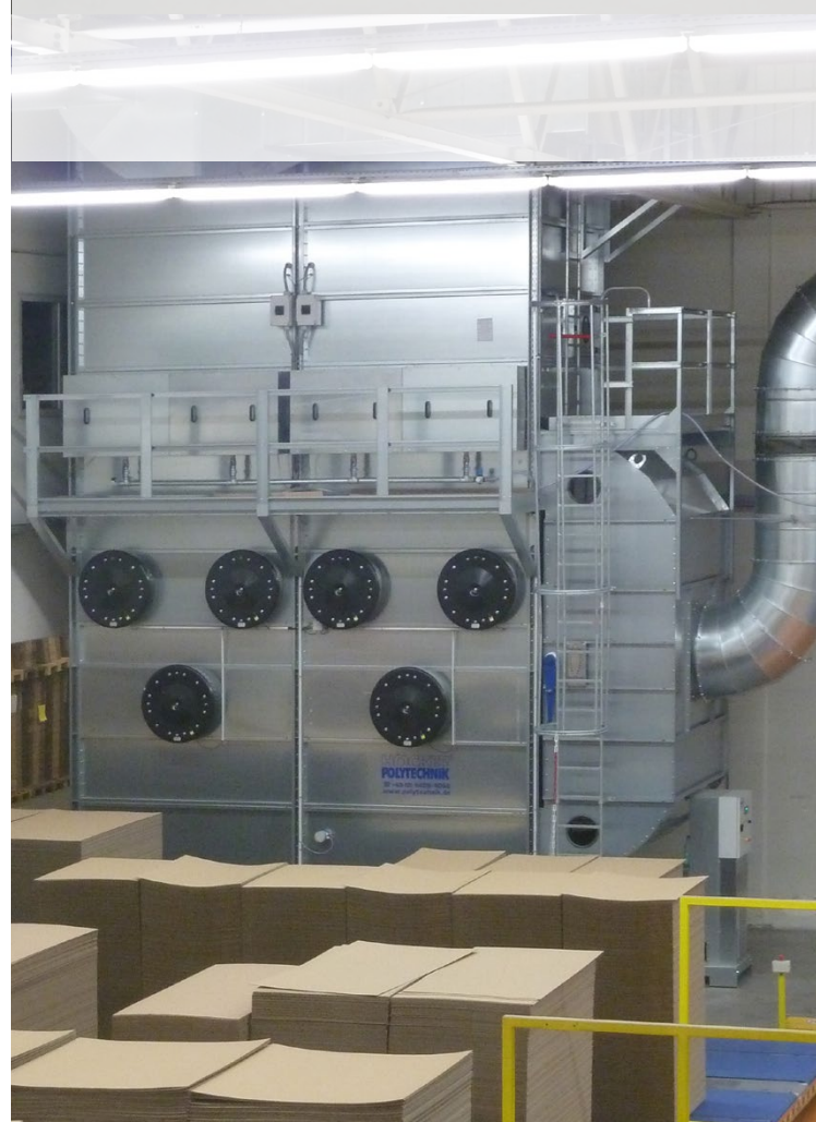
MultiStar jet filter in the packaging industry
